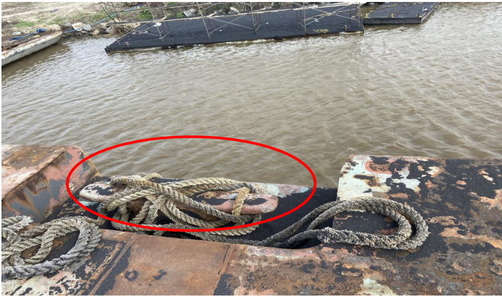
Figure 2. Photograph of cleat with mooring line secured to it on the top deck of the JMC 300; taken on February 10, 2024.
